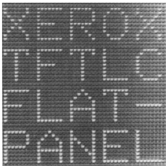
FIGURE 7 TFT-LC Panel with 2500 Elements, 1" × 1" size, Ref. 114. By permission of Fang-Chen Luo and the SID.
